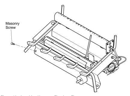
Figure 12 - Attaching Heater to Fireplace Floor
